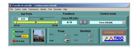
Control mode definition with transducer or calculated channel feedback selection.
